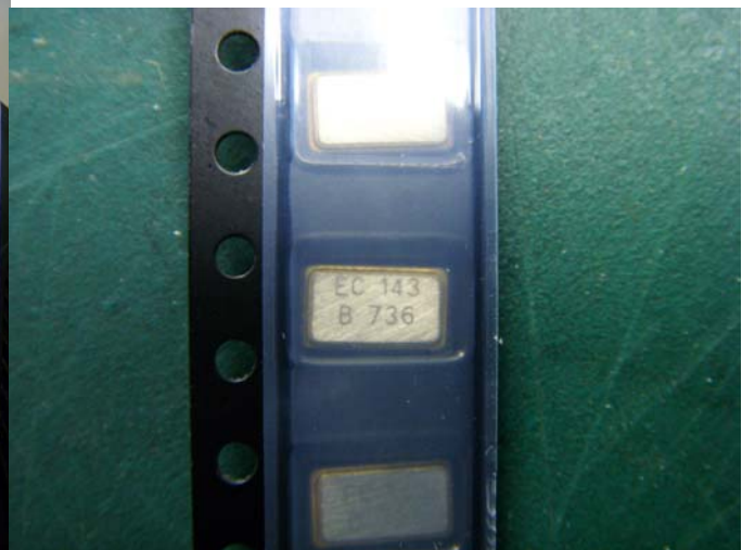
Photo 2) Counterfeit product that has been sanded and re-labeled.
