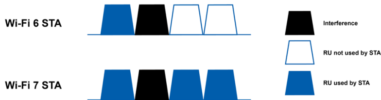
Fig. 4 gives a visual comparison of RU utilization between Wi-Fi 6 and Wi-Fi 7.
